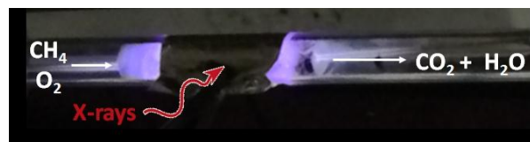
In situ XAFS set up to study, the NTP assisted CH_4 oxidation
