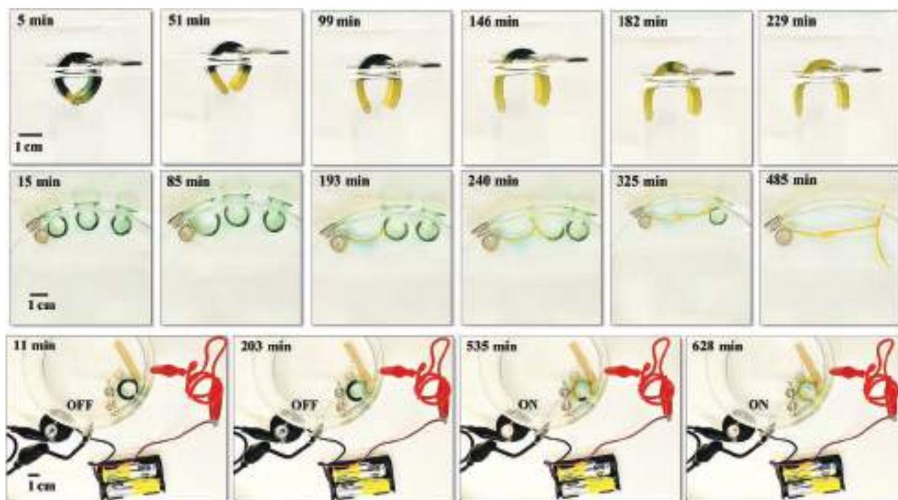
Figure 4. Experiments demonstrating the special features of hydrogels actuated by the autocatalytic front. From top to bottom: actuation in the air (100% humidity) of the hydrogel piece suspended on a spatula (autocatalysis was initiated from two sides of the hydrogel piece) (see also Video S6, Supporting Information); a relay system where actuation of one piece of hydrogel initiates the actuation of another (see also Video S7, Supporting Information); a delayed electrical switch created by actuating hydrogel (see also Video S8, Supporting Information). A thin copper wire was inserted into the hydrogel and contacted a brass plate when the hydrogel was actuated.
