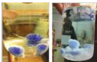
Fig. 6: (Colour online) Photographs of cellulose-titania hydrogels after squeezing out of a syringe Schweizer's reagent with a dissolved cellulose solution forming titania nanoparticles in the solution of \text{H}_2\text{SO}_4 . The blue hybrid still contains copper ions and amino groups. After several washings of the hybrid, it changes colour from bright blue to white, which is typical for a solely cellulose-based hybrid.
