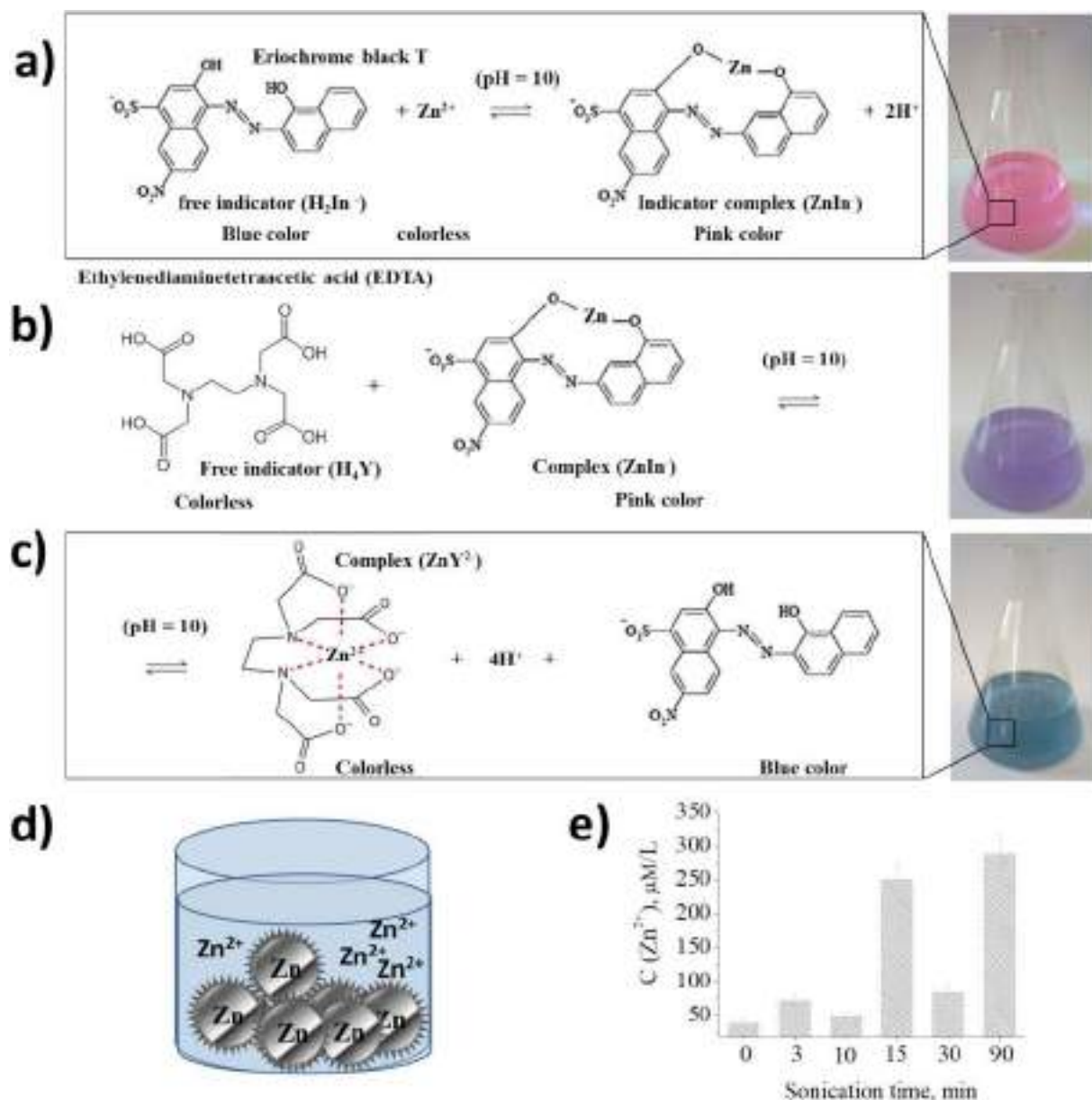
Fig. 4. The scheme of the reactions: a) between Zn^{2+} and eriochrome black T in water solution ( pH = 10 ); b–c) between ZnIn^- and Ethylenediaminetetraacetic acid (EDTA) in water solution ( pH = 10 ); d) schematic illustration of release experiment; e) the time dependence of concentration of Zn^{2+} ions leached from zinc particles treated sonochemically during different sonication time.
