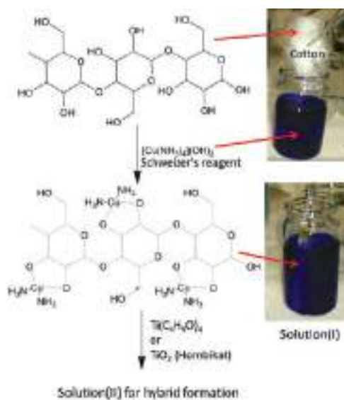
Fig. 2: (Colour online) Cellulose (white cotton fibres) dissolution in tetraaminecopper(II) hydroxide (Schweizer's reagent) for the formation of cellulose-based hybrids.
